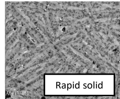
**Structure:** main - two phases: gray phase -  $\text{AB}_3$  ( $\text{LaNi}_3$ ,  $\text{La}_2\text{Ni}_7$ ), lighter dark phase -  $\text{LaNi}_5$ , impurity white phase - heavy phase with higher La content (possibly  $\text{La}_2\text{Ni}_3$ ). The study of the distribution of alloying elements (Co, Mn, Al) in alloys showed that the phases of type  $\text{AB}_3$  do not contain these elements, and they are concentrated mainly in the dark phase of  $\text{AB}_5$  type
