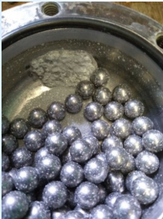
Photo of a lump formed in a mill by activated aluminum powder.
