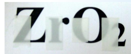
Films of different thickness: 80 \mu\text{m} , 160 \mu\text{m} and 320 \mu\text{m} (from left to right)
