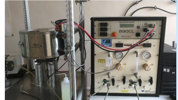
Photo and photomicrograph of a fuel cell made by tape casting; photo of the universal stand for testing fuel cells Scribner Teledyne Medusa RD 890CL
