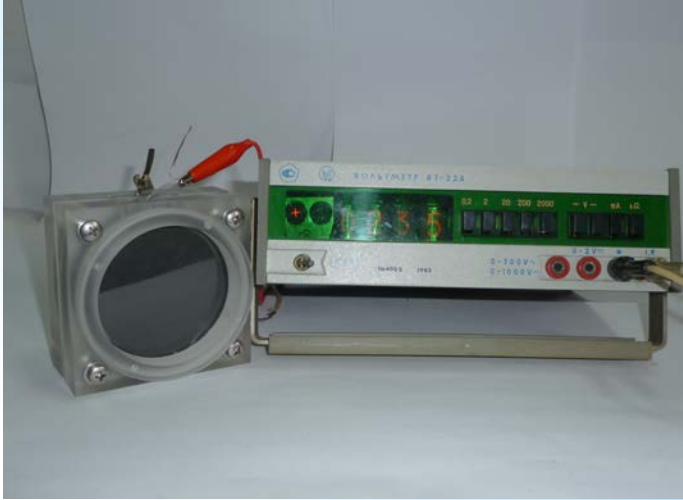
Electrochemical fuel cell with photoelectrode and MH / air electrode system.
