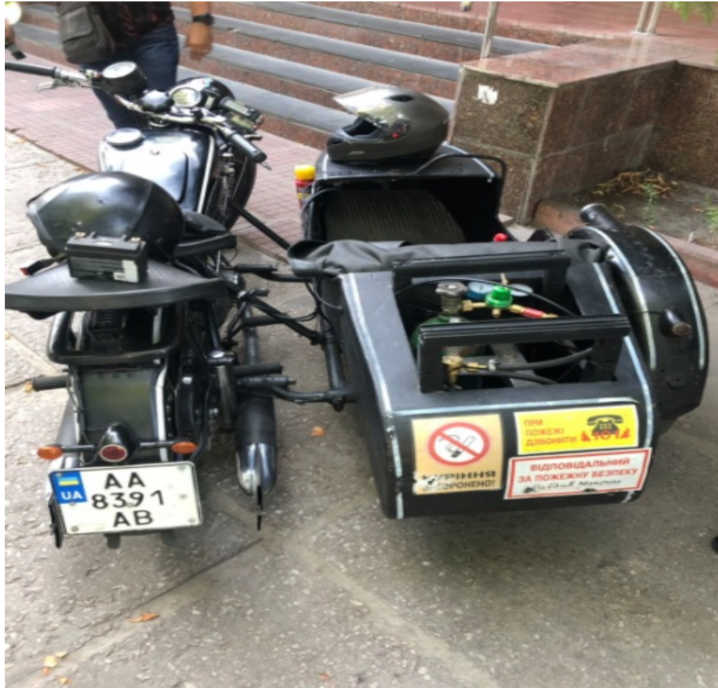
Motorcycle IZH-49, with a two-stroke engine 350 cm 3
