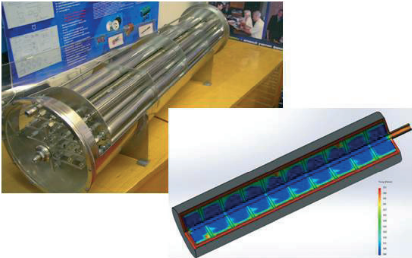
Fig. 3. Appearance and temperature field of a metal-hydride hydrogen storage system
