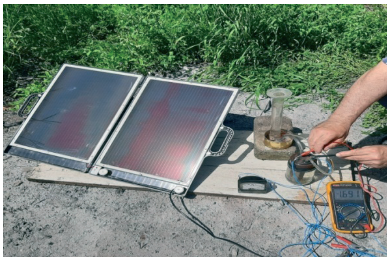
Fig. 1 The experimental laboratory installation with SPVC (TOPRAY SOLAR) in the real climatic conditions.
