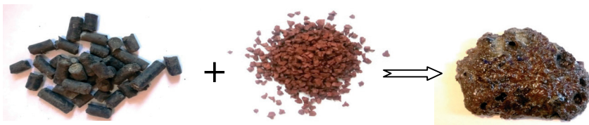
Fig. 4. Melt of slag (right), formed as a result of plasma-air gasification of sewage sludge (left) in a mixture with rubber roof of worn tires (middle)
