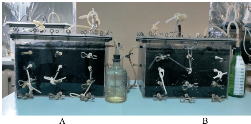
Fig. 5. Bioreactor-2 for purification of filtrate from fatty acids and alcohols: A- purification in anaerobic mode with \text{CH}_4 synthesis; B - purification in aerobic mode
