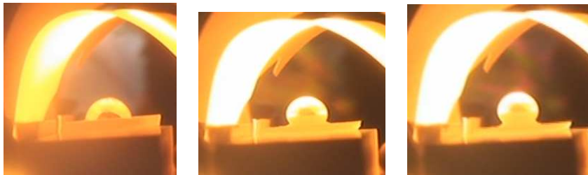
T = 900\text{ }^{\circ}\text{C}, \tau = 0:00, \theta = 60^{\circ} T = 1100\text{ }^{\circ}\text{C}, \tau = 0:05, \theta = 130^{\circ} T = 1250\text{ }^{\circ}\text{C}, \tau = 0:10, \theta = 150^{\circ} а б в
