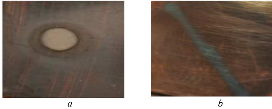
Fig. 7. Local coatings in the form of: a — spot; b — lines (x20).
