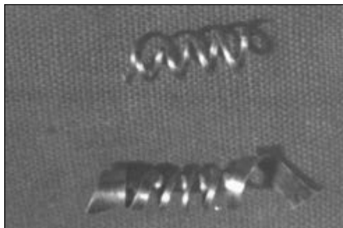
Fig. 8.15. Viscous fracture of the recrystallized Be—1.5Co after tensile testing at 1000K ( \times 600 )
