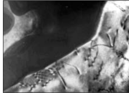
Fig. 11.3. Misfit dislocations at the interface of semi-coherent precipitates after the decomposition of \alpha -Mg solid solution
