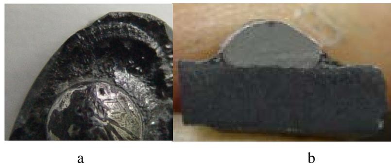
Fig.2. Sample after wetting experiment of rutile by iron: solidified drop (a) and its cross-section (b)
