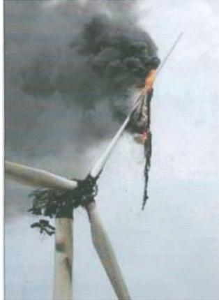
Fig. 1. Eventual pattern of destruction of wind power rotor blades
